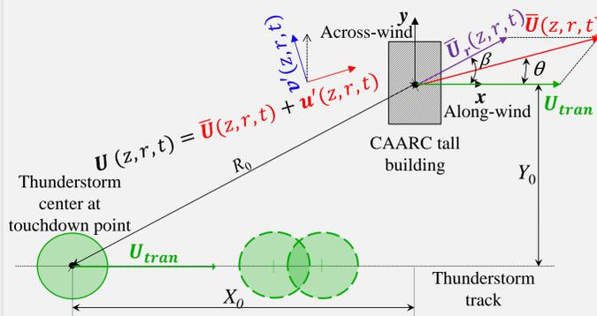
Schematic showing the placement of the structure with respect to the thunderstorm's path of travel
